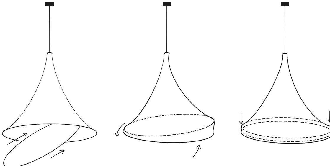
Insert the paper diffuser ring inside the textile shade as indicated in the figure.
